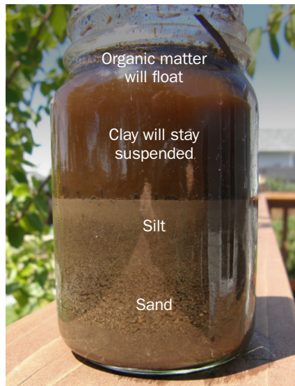
Figure 1: to determine your soil texture, perform a simple DIY texture test. BY CHERYL MOORE-GOUGH
